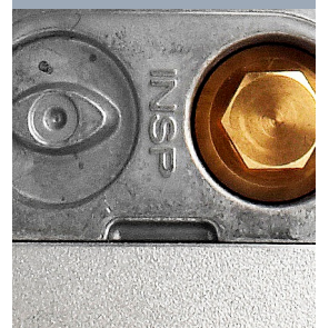
External oil and inspection plugs put an end to dismantling the entire pump to perform a simple seal-condition check and oil change.
