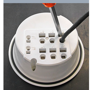
The watertight terminal board provides an additional barrier to water ingress. The spring-loaded, screwless design assures reliable connections and simplified wiring.
