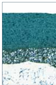
Cross section of Flygt epoxy coating
