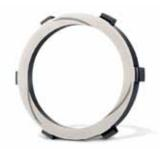
**ACTIVE SEAL™** technology from Flygt enhances sealing reliability by making the inner seal in a double seal system act as a micro pump. Laser-cut spiral grooves in the seal face of the inner seal pump liquid from the inner to the outer diameter of the seal ring, thus preventing liquid from entering the stator housing.
